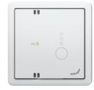
The Zehnder 12V 0-10V remote CO2 sensor and combined three position switch is designed to enable the user to manually select the desired ventilation systems flow rate based on the visual air quality indicator, or automatically adjust the unit relevant to the CO2 level.
